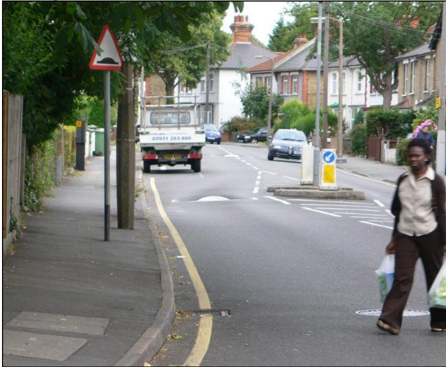
Fig 5. Oakhill Road by the junction with the High Street. 'Road-hump' signage clutter reduces the usable width of the already narrow pavement, and a crossing situated away from the desire line is ignored.
