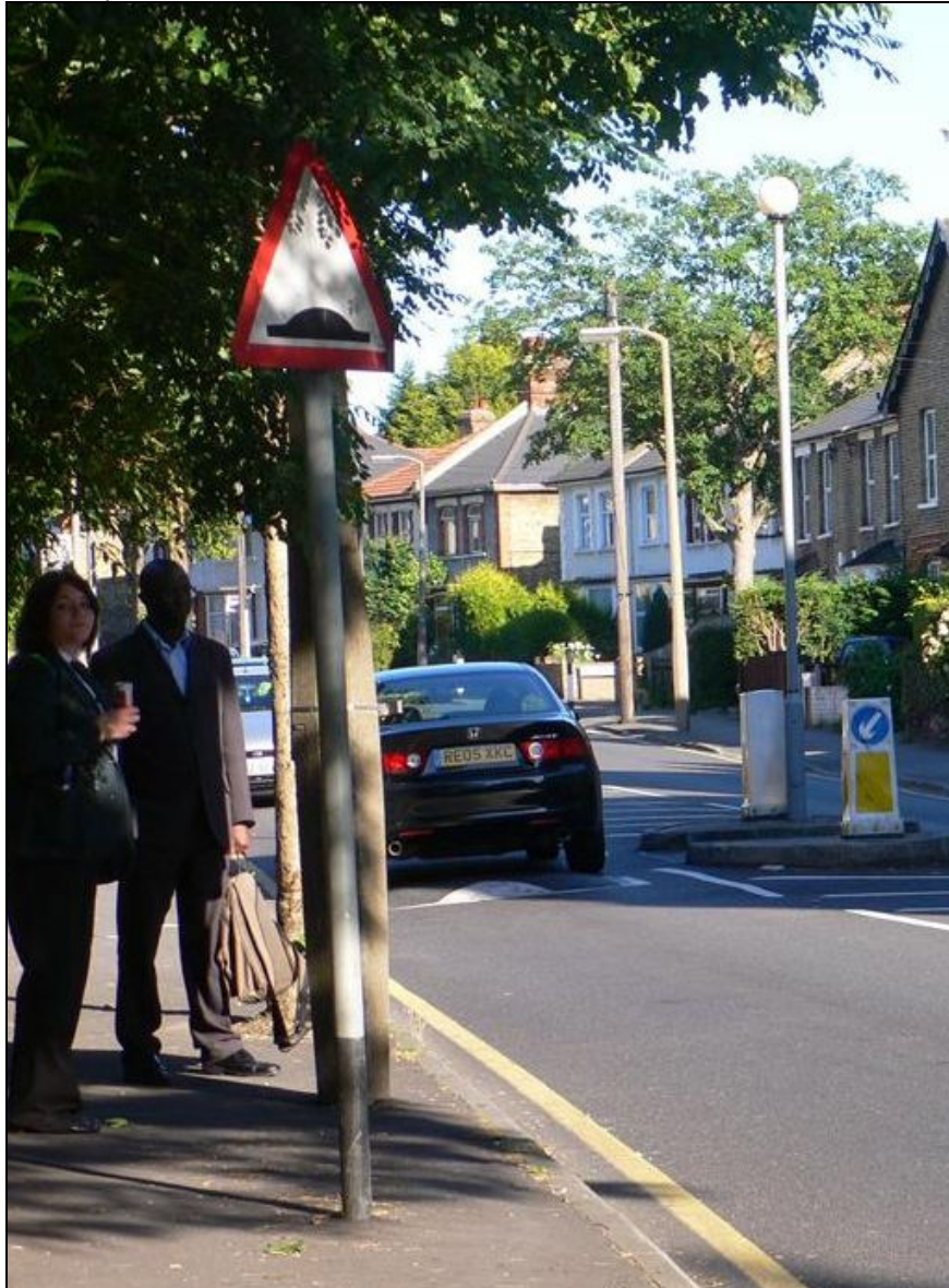
Fig 4. Oakhill Road near junction with High Street. A dilemma! Road-humps need signs, but road-hump signs can block the pavement!
